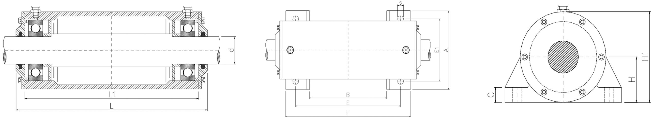
These housings are especially suitable for ventilation fans running with a higher speed than common pillow blocks. Since misalignment errors are largely excluded, ball bearings can be installed in these housings. The grease quantity control discs on both sides simplify maintenance and throw excess grease into the middle of the large housing space.
